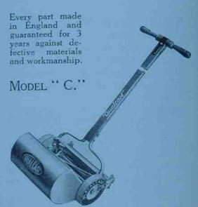
SPECIFICATION.—Driving wheels 7ins. diam. by 11/4in. tread, Cutting Cylinder 5in, diam. fitted with 5 blades best Sheffield Steel. Lip edge section bottom blade, Spanner supplied which fits all nuts, Attractively finished in Qualcast Blue and each machine packed in a separate box. Note.—The 12in. and 14in, machines are fitted with Bronze Bearings.
