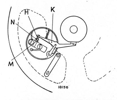
CONTACT BREAKER. TWO STROKE MODEL.
