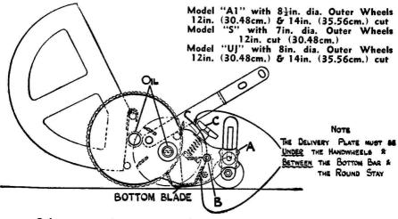
Before commencing to cut, see that the Lawn Mower is clean, then oil all the bearings in the holes provided, with the best machine oil, at the same time putting a little on the edges of all the cutters and bottom blade, and secure the handle firmly in the socket.
