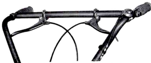
View showing assembly position of clutch controls. Transferred on to cross member. This control arrangement is more convenient when trailer is used.
