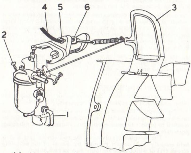
(g) After the engine has started, gradually open strangler as engine warms up. When engine is warm and running smoothly, partially close control lever so that engine is idling.
