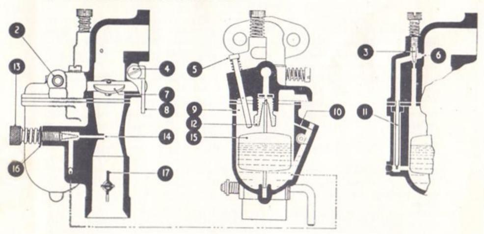
The 13TCA-2 carburetter shown above has a high non-flooding angle in all directions, and consists of two principal castings. The upper portion or throttle body incorporates the right angle inlet bend and the fixing flange which is bolted directly on to the inlet port of cylinder: the lower portion consists of the float chamber (or bowl) and the air intake. The choke tube is cast integrally as part of the air intake.
